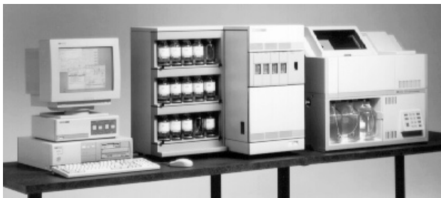
Fig. 5. The HP G1009A C-terminal protein sequencing system consists of the HP C-terminal sequencer, the HP 1090M HPLC, and an HP Vectra computer.
